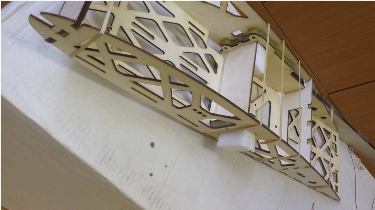
Figure 3.11. Gluing of the nacelle
