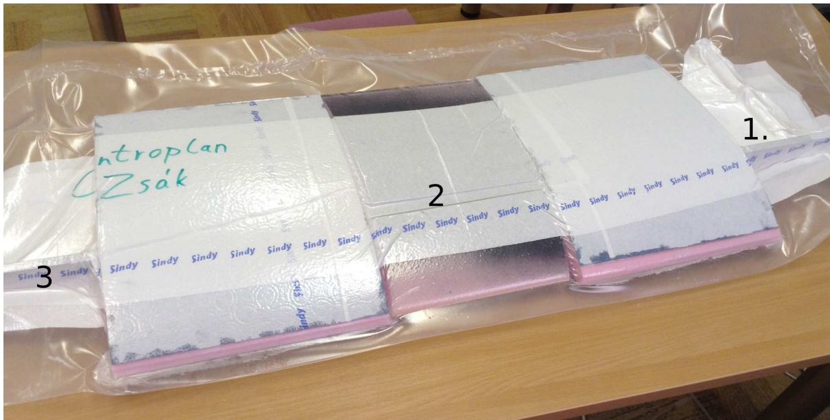
Figure 6.3. Vacuum bag for the central wing sections
