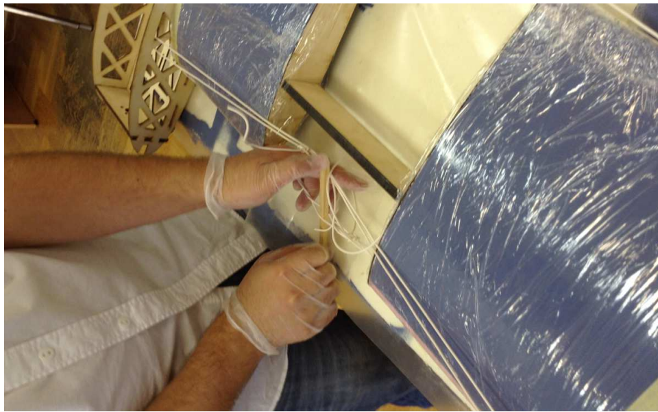
Figure 7.3. Squeezing nacelles during epoxy curing
