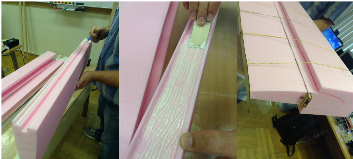
Figure 5.9. Gluing in the spar
