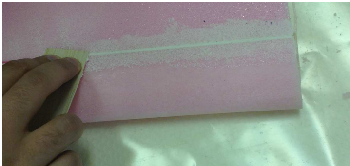
Figure 5.17. Filling the gap with filler mixed epoxy
