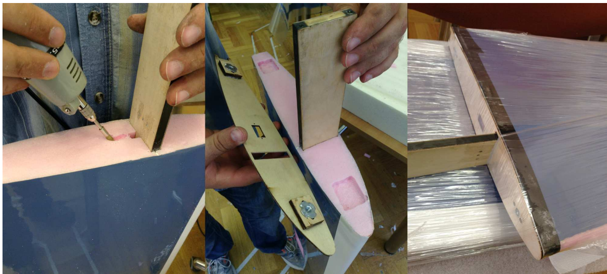
Figure 7.8. Gluing in the connecting parts
