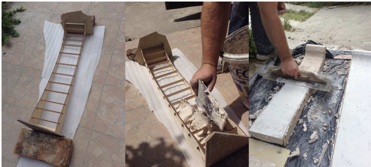
Figure 4.4. Filling the plaster into the container
