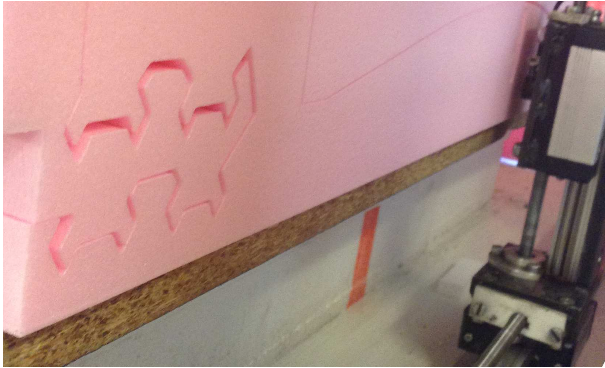
Figure 5.4. Kerf calibration in practice
