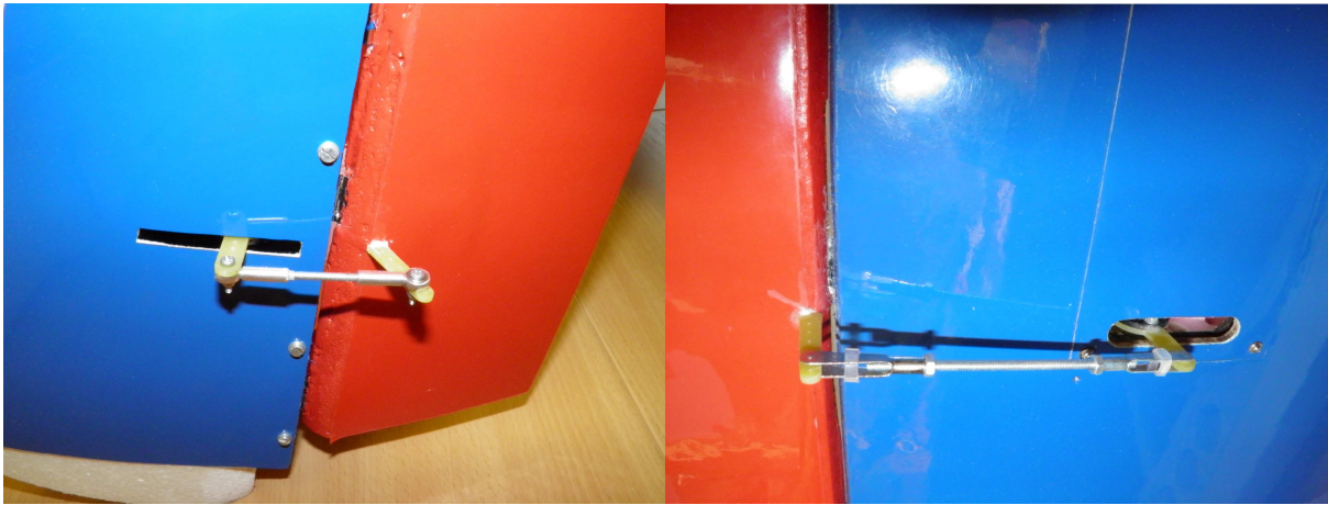
Figure 7.20. Servo rods on the rudder (left) and aileron (right)
