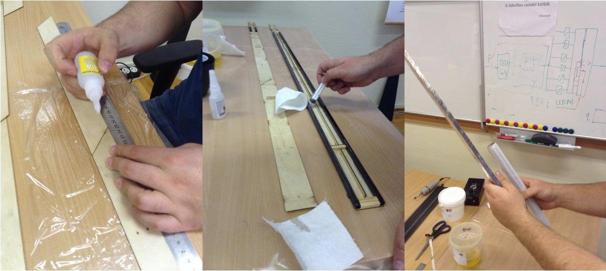
Figure 2.4. Steps of a spar assembly
