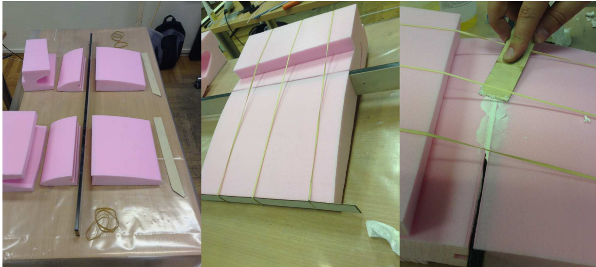
Figure 5.13. Gluing the spar and filling the gaps
